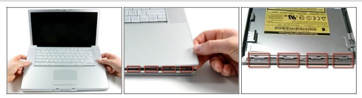
Do not yank the upper case off quickly. The case is attached to the logic board via a ribbon cable.
